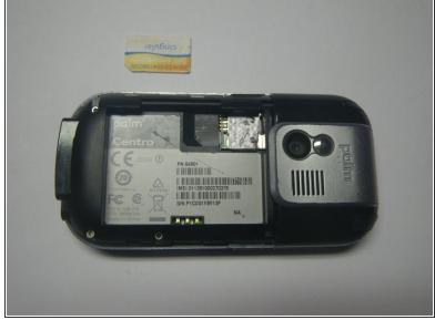
Remove the SIM card so housing can be separated.
