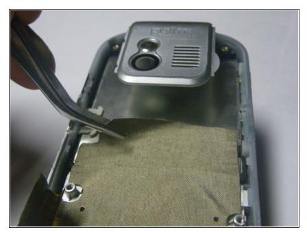
Slowly peel off the protective lining that is on the screen and keyboard.
