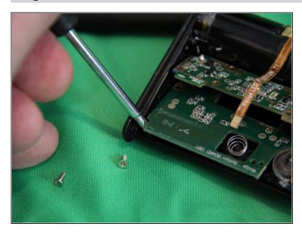
Insert a small flat blade screw driver as shown and gently pry the lower PCB out from under the plastic retaining clip.
