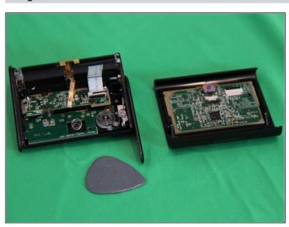
Push down upper PCB, reinsert and tighten the 2 black screws, if you removed all 4 during disassembly, remember to put the lens and iris back under the upper PCB before pushing it down and tightening all 4 black screws.
