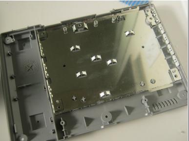
Reinstall the RF shield by dropping it in and lining up the slots and tabs.
