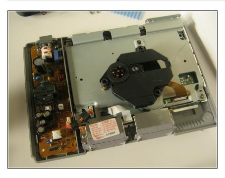
Turn the unit back over, and pull the top half up and away from the device.
