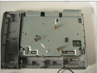
Remove the 3 screws from the shield.
