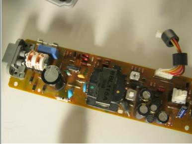
To remove the power supply, disconnect the cable and remove the two screws, then lift it out of the case.
