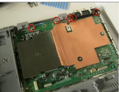
Replace the main board. Only install the screws indicated in red.
