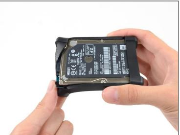
• Peel the flexible hard drive sleeve off the top left corner of the hard drive.
