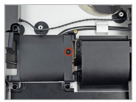
Remove the single 7.2 mm T10 screw securing the hard drive tray to the rear enclosure.
