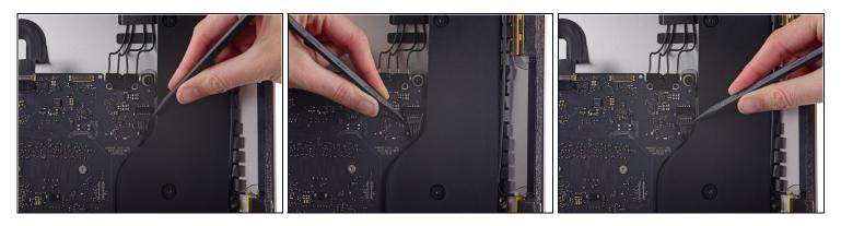
• Use the tip of a spudger to push on either side of the right speaker cable connector to *walk* it out of its socket on the logic board.
