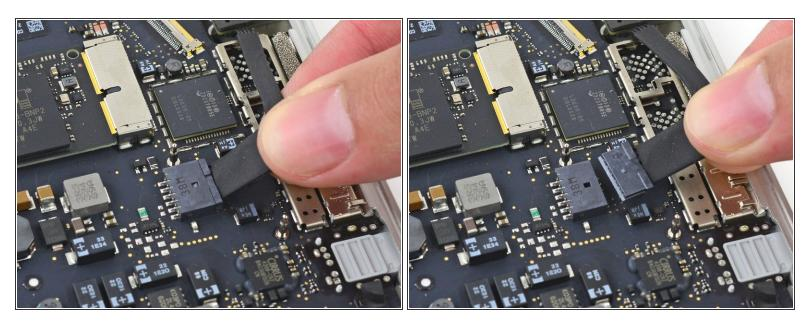
• Pull the DC-In board connector straight out of its socket on the logic board.
