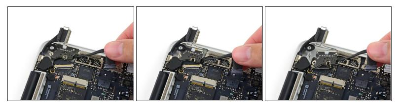
• Use the MagSafe DC-In board cable to pull the board out and up from the upper case to remove it.
