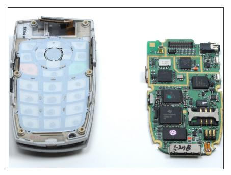
Once the ribbon is detached, remove the logic board and replace if necessary.
