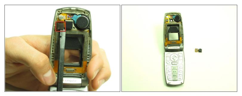
Use a spudger to pop off the camera ribbon from the main ribbon. The camera component should separate entirely.
