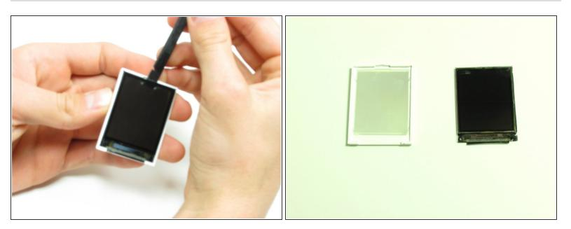
• Use the spudger to remove the LCD screen from its backing.
