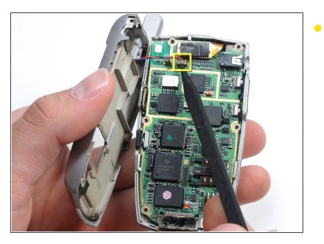
Use a spudger to disconnect antenna wire.
