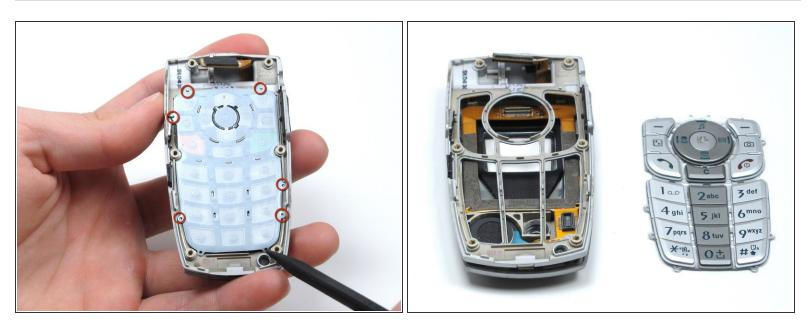
Using a spudger, lift the keypad off of the tabs.
