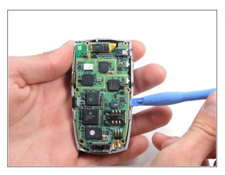
• Use the IPod opening tool to pop out the logic board.
