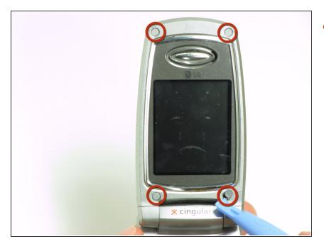
Remove all four screw covers by using an IPod opening tool. They should come off relatively easy.
