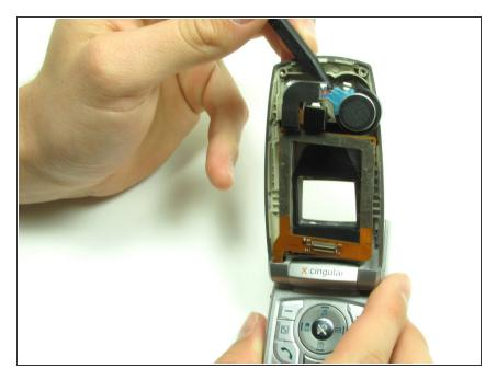
• Carefully slide the spudger behind the main ribbon in order to separate it from the inside cover of the phone.
