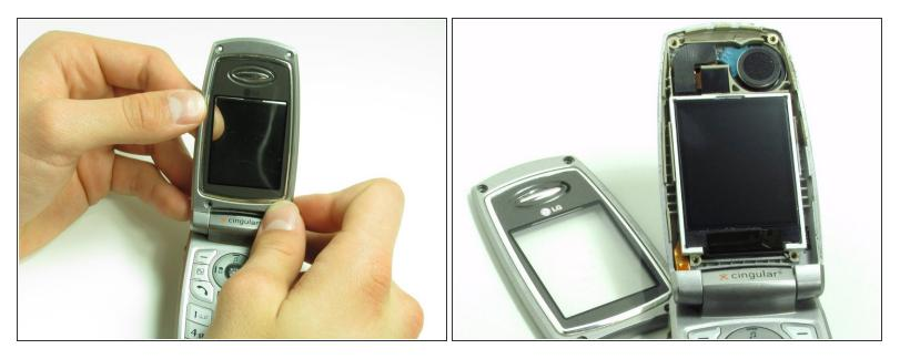
• Pull the inner screen cover towards you and up in order to separate it from the front cover.
