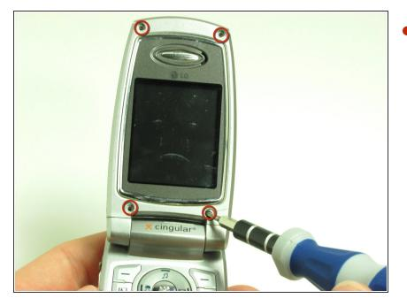
Using a T6 Torx screwdriver, remove all four screws.
