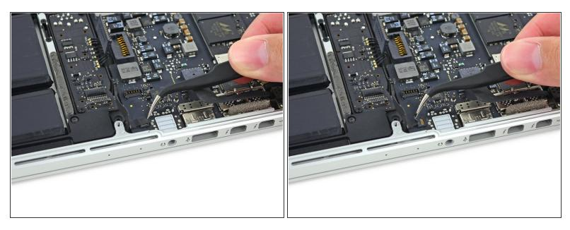
(i) If necessary, peel back any tape covering the microphone cable ZIF connector.
