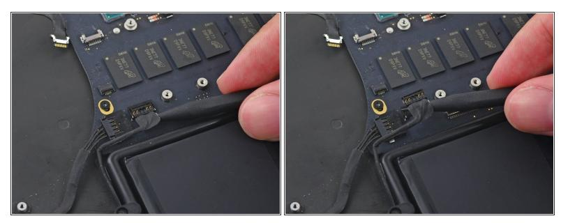
Use the tip of a spudger to lift the right speaker connector straight up out of its socket on the logic board.
