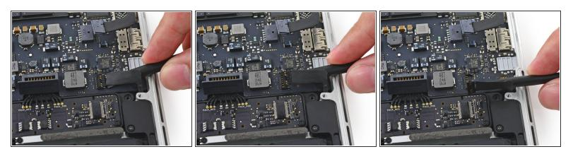
• Wedge the flat end of a spudger under the left speaker cable near the connector and lift it straight up out of its socket and fold it out of the way.
