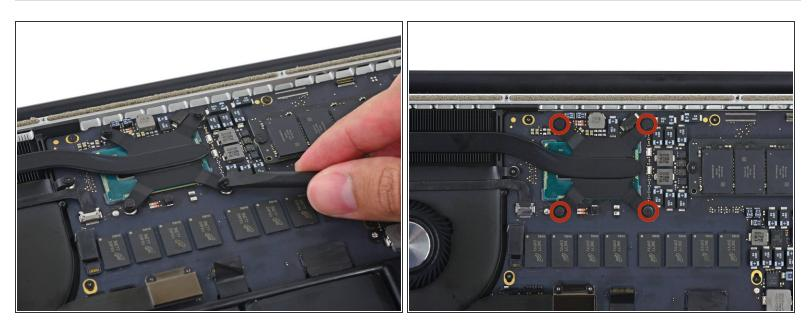
• Use the flat end of a spudger to peel the four foam stickers off of the heat sink screws.
