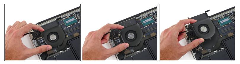
• Lift the end of the fan closest to the display hinge and remove the fan from the upper case.
