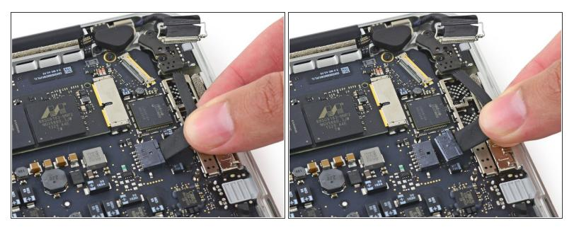
• Carefully pull the DC-In board connector straight out of its socket on the logic board.
