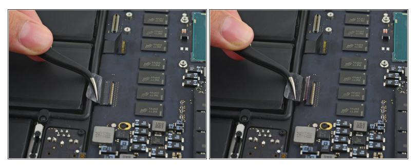
• Pull the keyboard cable straight out of its ZIF socket on the logic board.
