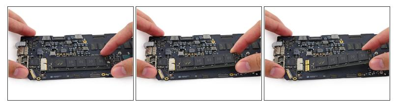
• Lift the free end of the SSD up slightly and pull it straight out of its socket on the logic board.
