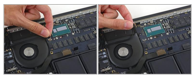
• Peel the iSight camera cable off the fan housing to fold it out of the way.
