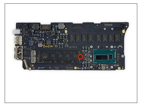
Remove the single 2.9 mm T5 Torx screw securing the SSD to the logic board.
