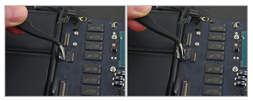
• Pull the trackpad ribbon cable straight out of its socket on the logic board.
