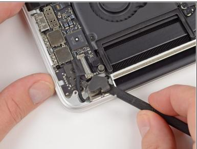
Use the flat end of a spudger to pry off the two rubber hinge covers, one from each end of the device.
