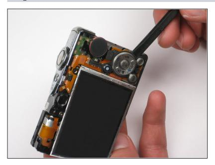
Remove the function buttons by sliding the spudger underneath the black rubber and lifting up.
