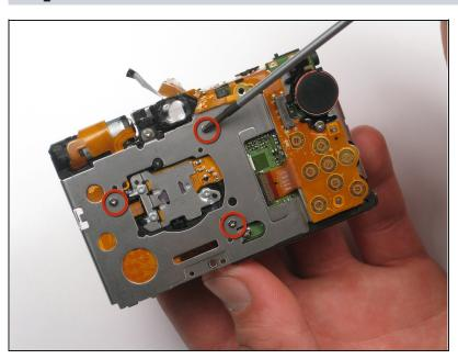
Remove the three screws which secure the lens assembly to the main chassis.
