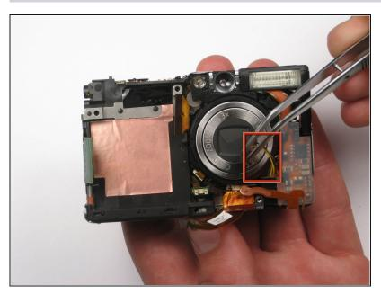
Grasp the plug that yellow and black wires are attached to, and gently remove. <u>Tweezers</u> are very helpful here.
