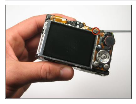
Remove the screw at the upper right-hand corner of the LCD screen
