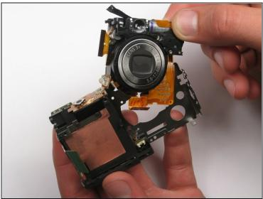
• Remove the lens carefully from the chassis. You're done!
