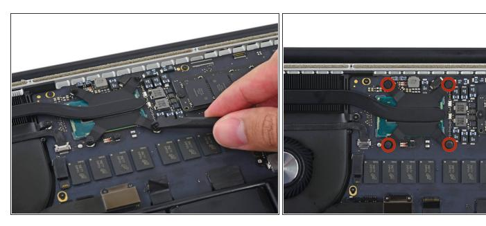
Use the flat end of a spudger to peel the four foam stickers off of the heat sink screws.
