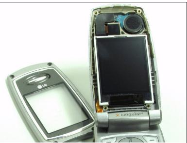
Pull the inner screen cover towards you and up in order to separate it from the front cover.
