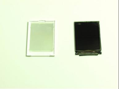
Use the spudger to remove the LCD screen from its backing.
