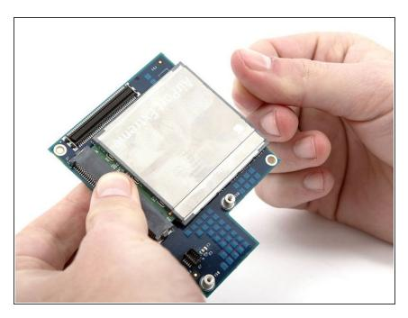
Grasp the wireless interface board with one hand and the clear plastic tab on the Airport card with the other hand, and pull the Airport from its connector.
