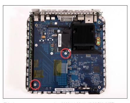
Remove the two silver Phillips screws from the corners of the wireless interface board.
