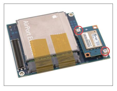
Remove the two silver Phillips screws from the corners of the Bluetooth board.
