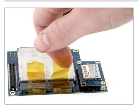
Remove the yellow tape securing the Airport card to the wireless interface board.
