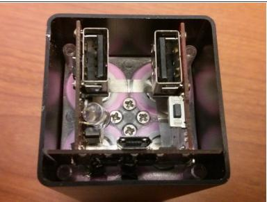
Remove 4 Philips screws to release the plastic cover
