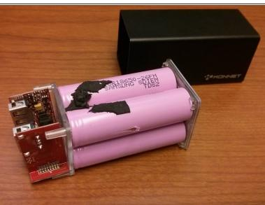
Carefully push from the side you just opened. All the inside parts should slide out from the back of the unit.
