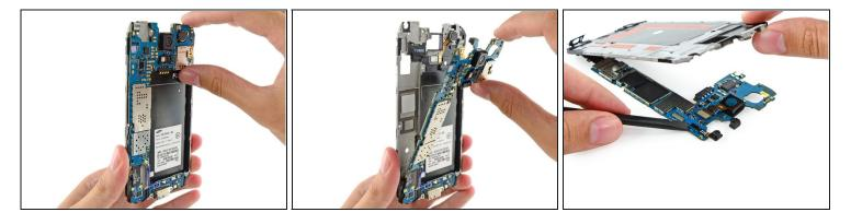
• Pull, but do **not** remove, the motherboard away from the midframe to allow access to the connectors on the rear.
