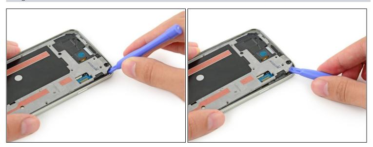
• Use a plastic opening tool to pry any remaining corners out of the silver bezel.
