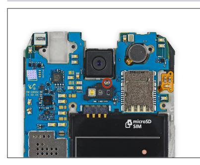
• Remove the single 3.0 mm Phillips #00 screw securing the motherboard to the midframe.
