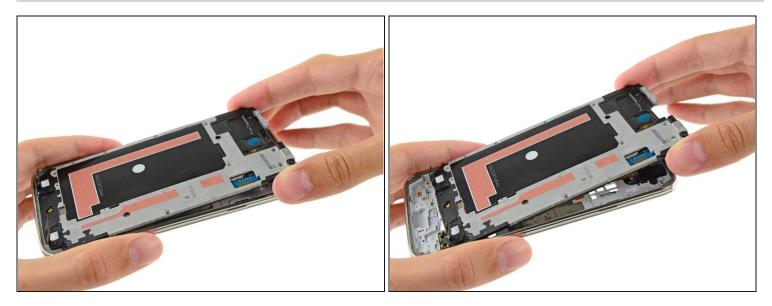
• Carefully remove the interior midframe/motherboard assembly from the white inner midframe.
