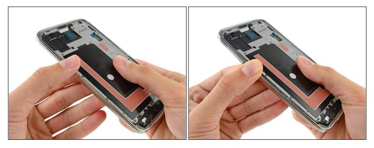
(*i*) The midframe is composed of two halves that encase the motherboard.
