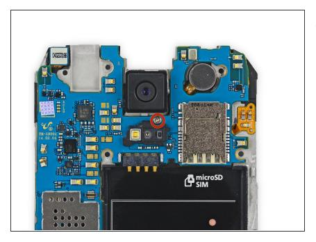
Remove the single 3.0 mm Phillips #00 screw securing the motherboard to the midframe.
