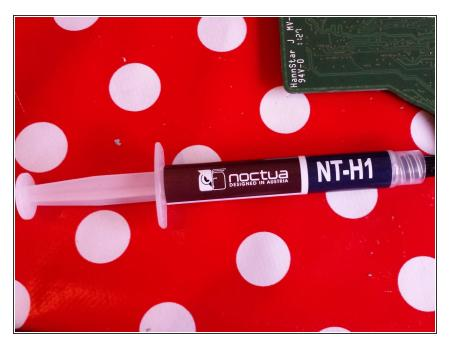
This is time to replace the old paste with a new one. Buy a good quality paste to ensure a proper heat dissipation.
