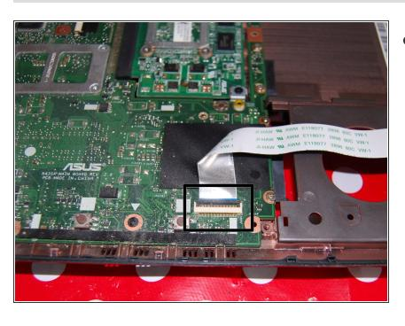
Remove this cable the same way than the step 9 and 10.
