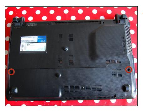
Remove the two philips screws from the cover.
