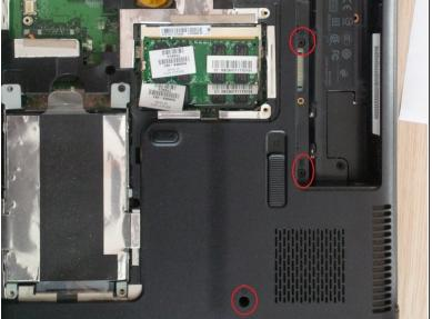
Remove the screws to remove the keyboard.
