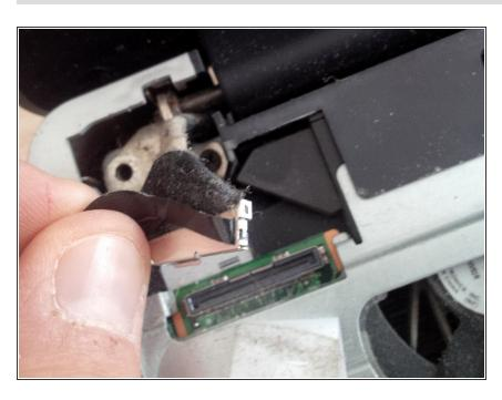
Remove the black flat wire of the LCD screen from the motherboard.
