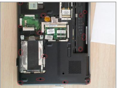
Remove the screws that are circled in the picture. These screws hold the case of the laptop.
