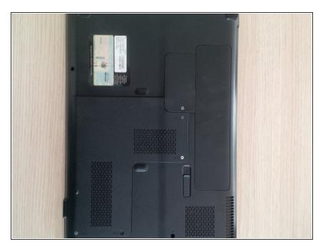
Turn the device over and remove the screws from the battery.
