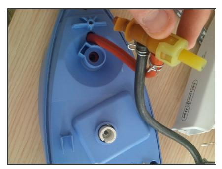
remove the blue bottom plate and the cables
