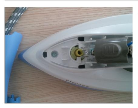
remove the screw at the pointed side of the iron.
