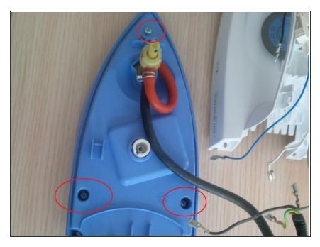
remove the bottom plate screws.
