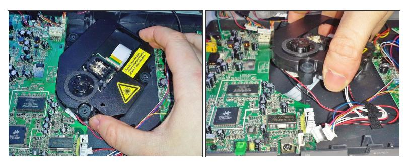
Remove the optical disc drive by lifting it off the three pegs on the bottom case.
