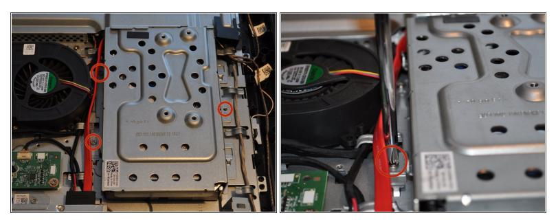
• Remove the three screws that hold the hard drive cage to the chassis.
