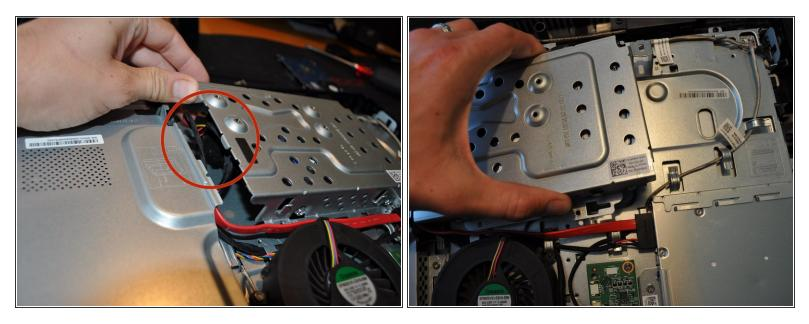
• Slide the hard drive cage out slightly to access and remove the power and SATA cable.
