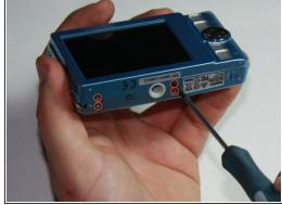
Remove the eight screws around the sides and bottom of the camera using a Phillips #00 screwdriver.
