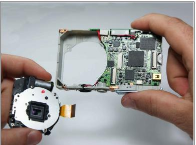
Carefully unplug the golden wire from the motherboard to remove the lens from the assembly.
