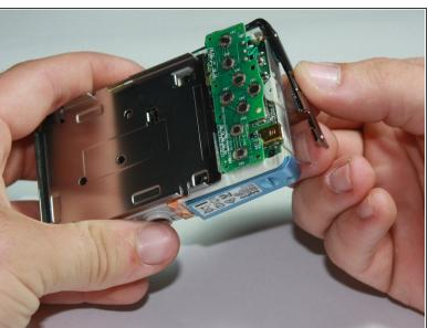
Carefully pull off the side covers wrapped around the camera.
