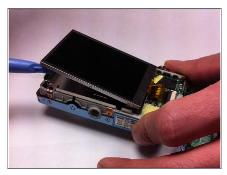
The LCD screen should now be disconnected from the rest of the camera and a pry tool can be used to lift it out of its casing.
