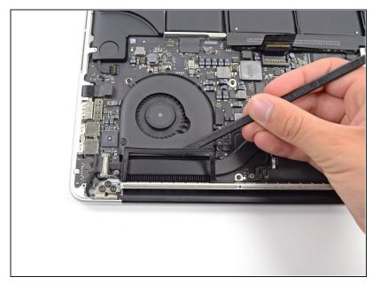
Use the flat end of a spudger to lift the rubber heat sink cover up off the left fan.
