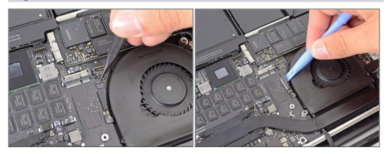
• Use the tip of a spudger to flip up the retaining flap on the right fan ribbon cable **ZIF** socket.
