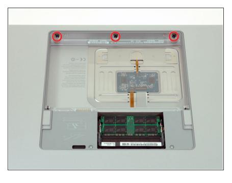
Remove the three Phillips screws in the battery compartment near the latch. Apple was nice enough to tilt these screws at a slight angle to make them easier to remove. On the A1261 these screws have 4 mm diameter heads rather than the 3 mm heads on the body screws.
