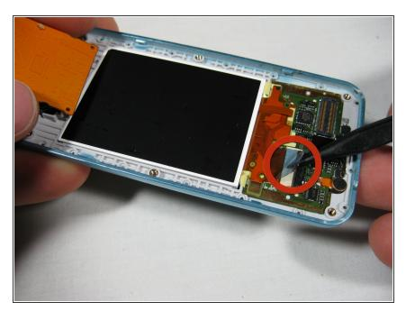
Lift and remove the blue tape from screen connector.
