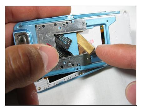
Slide ribbon cable through the slider mechanism.
