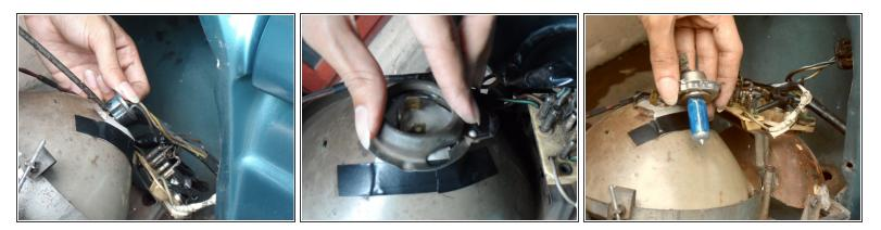
• Carefully unplug the headlamp socket, and then rotate the metal ring, which holds the bulb to the body. Then, pull the bulb out slowly.
