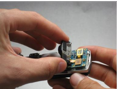
Use the iFixit opening tool to remove the camera/speaker from the motherboard.
