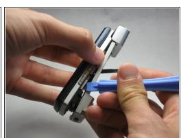
Locate the USB port (where the charger can be plugged in). Using the iFixit opening tool, open the phone cover.
