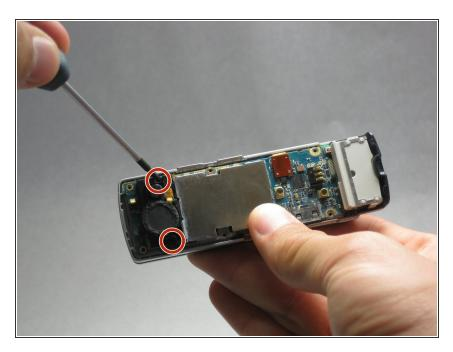
Remove the 5.5 mm screws from both sides of the camera/speaker with a Phillips #00 screwdriver.
