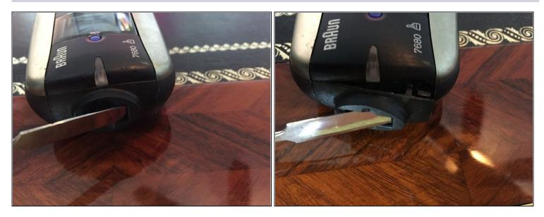
• First pry the left side of the cover off, then pry the right side of the cover off before removing. Trying to pry the cover off from only one side will result in breaking the plastic tabs.
