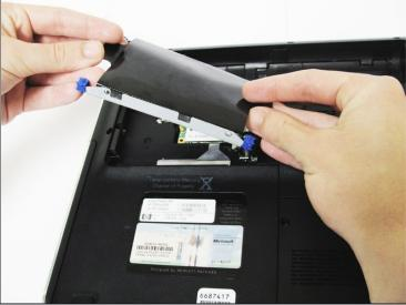
• Pull up on the two plastic flaps on the hard drive enclosure to remove it.
