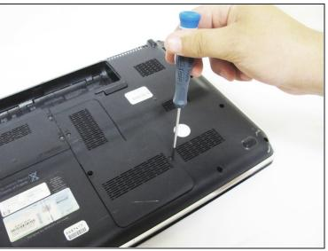
Remove these two 4mm Phillips screws on the back panel using a Phillips #00 screwdriver and remove the cover to reveal the CMOS battery
