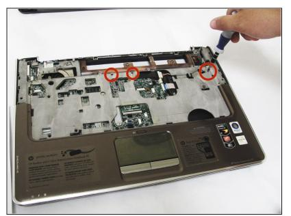
Remove the three 3mm Phillips head screws on the top of the frame using the Phillips #00 screwdriver.
