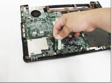
• Using the Phillips #00 screwdriver, unscrew the spring-release fasteners on the modem card and remove it from the board.
