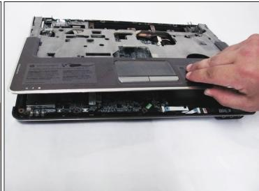
• Using a plastic opening tool, carefully pry off the top plastic cover by lifting it up at the seam at various points around the edge, then remove it completely.
