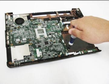
• Remove the two 2mm screws on the bottom right of the motherboard using the Phillips #00 screwdriver.
