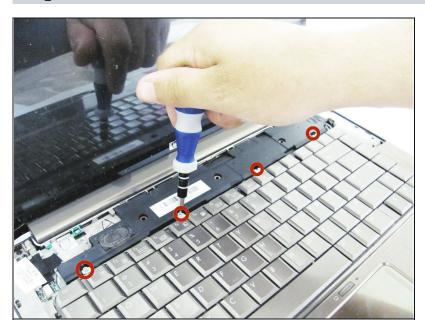
Use a 2.5mm flathead screwdriver to remove the four 3mm screws on top of the keyboard.
