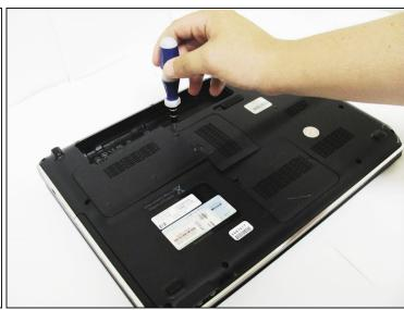
• Remove the two 5mm Phillips screws on the hard drive cover using a Phillips #00 screwdriver.
