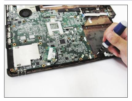
Remove the one 3mm Phillips screw on the bottom left corner of the board using the Phillips #00 Screwdriver.
