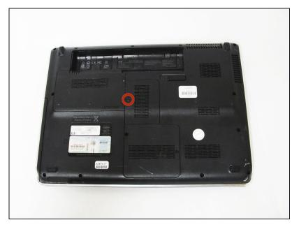
Remove the one 4mm Phillips screw from the RAM cover using a Phillips #00 screwdriver.
