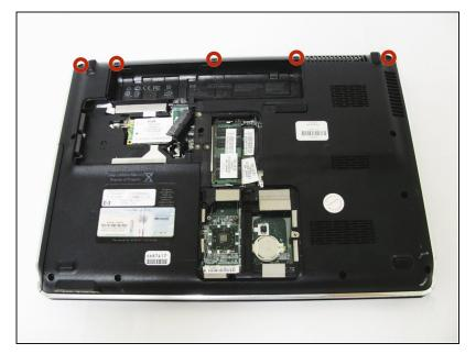
Remove the five remaining 2mm screws using a Phillips #00 screwdriver.
