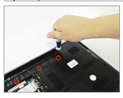
Begin by unscrewing the three 3mm Phillips head screws inside the battery bay with the Phillips #00 screwdriver.
