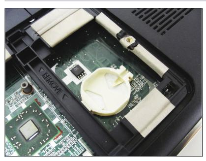
• The CMOS battery is now removed from your system.
