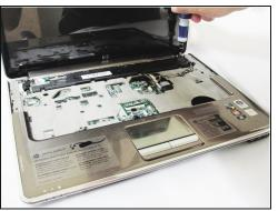
• Locate four 3mm screws in the upper corners of the keyboard tray and remove them using a #00 Phillips screwdriver.
