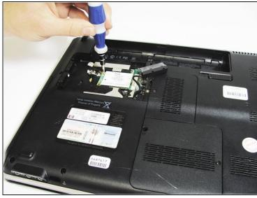
• Locate the 2.5mm Phillips screw on the corner of the WLAN card and remove it using a Phillips #000 screwdriver.
