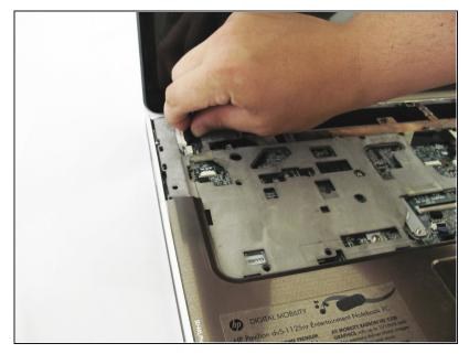
Locate the large display ribbon connector near the upper left corner of the keyboard tray and remove the ribbon by pulling straight out on the connector.
