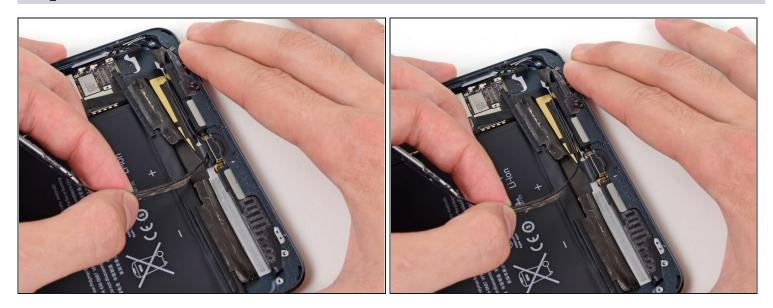
• Pull the antenna cable from the slot behind the Lightning connector.
