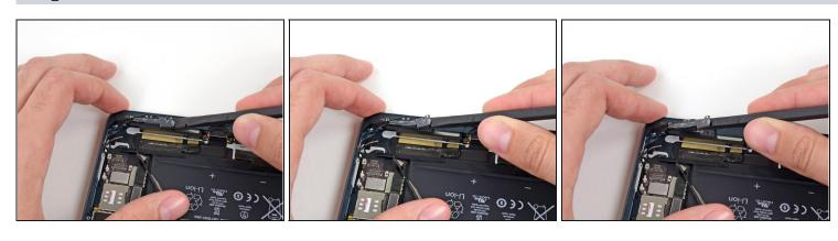
• Use the flat end of a spudger to loosen the foam adhesive holding the GPS antenna to the right speaker.
