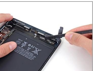
• Use the flat end of a spudger to fold the left-hand wide piece of tape away from the left speaker.
