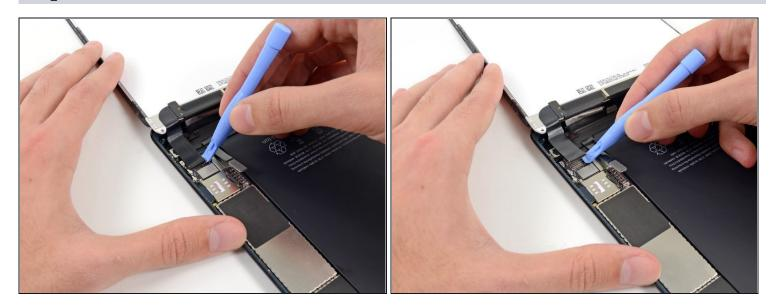
• Use a plastic opening tool to pry the LCD connector from its socket on the logic board.
