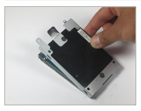
Access to the Hard drive by gently sliding the metal cover away from the Hard Drive.
