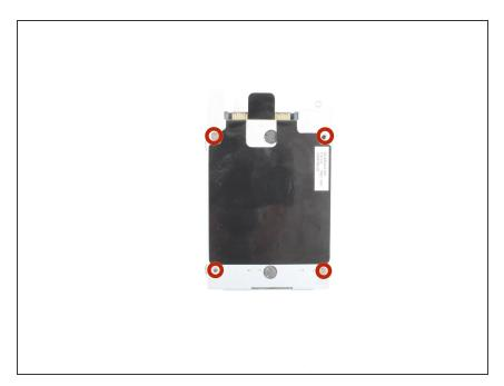
Remove the four identical 1/8" Phillip screws located in every corner of the Hard Drive using the Phillips #0 Screwdriver.
