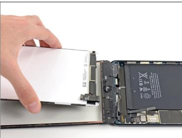
• Lift and remove the LCD from the iPad Mini.
