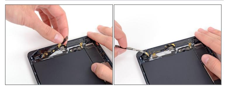
Lift the headphone jack cable up and fold it out of the way.
