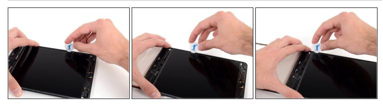
• Insert the guitar pick into three more locations down the left side of the LCD and bend it over in each location, to slide the LCD over to the right side of the rear case.
