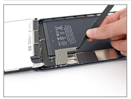
Use a pair of tweezers to grasp and remove the connector shield from the iPad.
