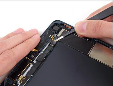
Use a pair of tweezers to peel up and remove the small piece of tape covering the front-facing camera cable connector.
