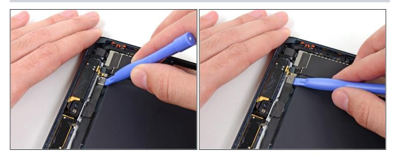
Use a plastic opening tool to pry the front-facing camera cable's connector up from its socket on the logic board.
