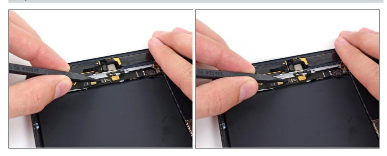
Use the tip of a spudger to lift the tab on the microphone data cable ZIF connector.
