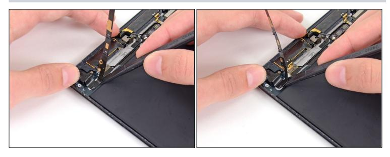
• Use the flat end of a spudger to pry the headphone jack cable up from the adhesive securing it to the rear case.
