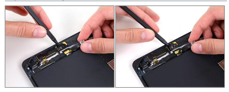
• Use the tip of a spudger to gently pry the front-facing camera forward, separating it from the adhesive securing to the rear case.
