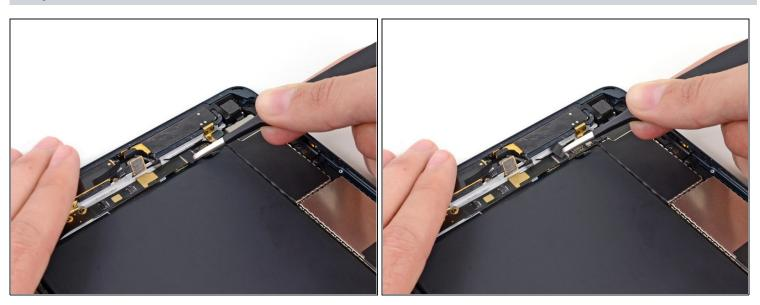
Peel up and remove the small piece of tape covering the headphone jack cable connector.
