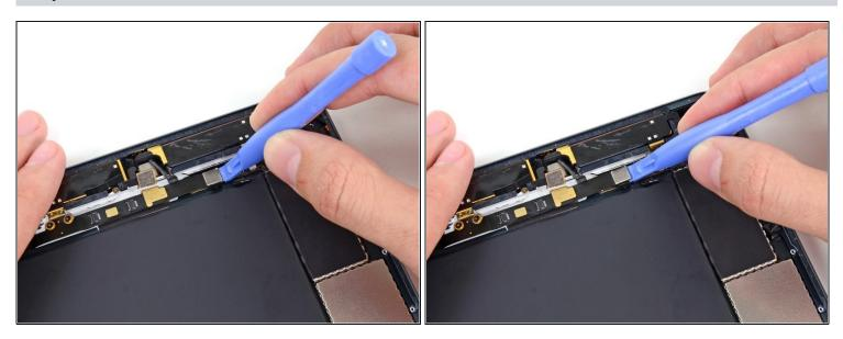
• Use a plastic opening tool to pry the headphone cable's connector up from the logic board.
