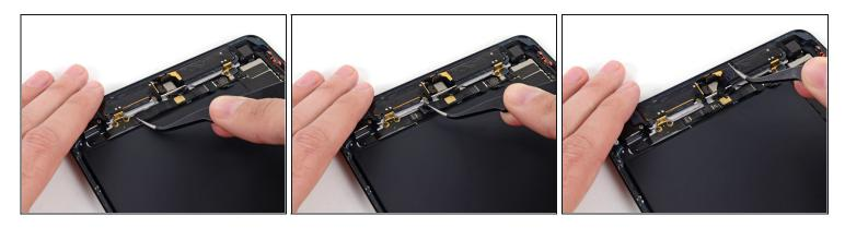
Use tweezers to peel and remove the long thin black tape covering the top of the headphone jack cable.
