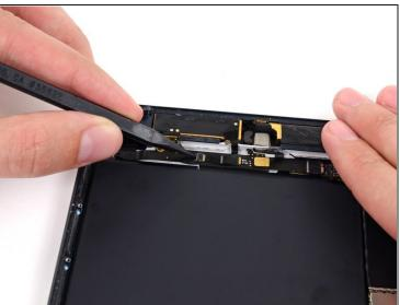
Use the tip of a spudger to gently lift the tab on the top left antenna ribbon cable's ZIF connector.
