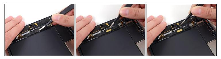
• Use a pair of tweezers to peel up the top of the rectangular piece of tape covering the bend in the front-facing camera cable.
