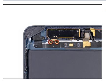
Remove two 1.8 mm #00 Phillips screws from the screw tab on the top left antenna.
