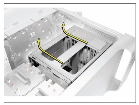
Slide the memory cage and fan toward the power supply far enough that the cage clears the bottom edge of the enclosure. Then lift the memory cage and fan out of the enclosure.
