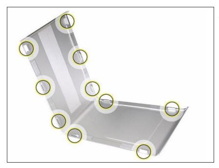
Replacement Note: When reinstalling the processor heatsink cover, make sure the tabs on the underside of the cover align with the slots directly below them. (The slots are on the front fan and memory cage on either side of the heatsink cover.)
