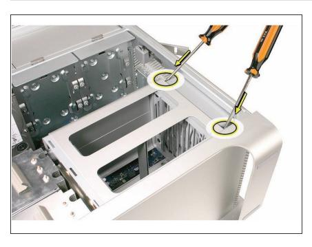
Using a flat-blade screwdriver, release the two latches nearest the front of the computer.
