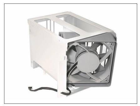
installing a new fan in the memory cage assembly, rotate the fan into the cage as illustrated. Also note carefully the orientation of the fan in relation to the cage.
