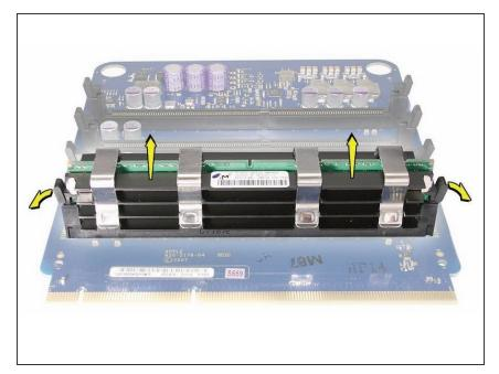
Open the ejectors on the DIMM slot by pushing them out to the sides, and remove the DIMM from the riser card.
