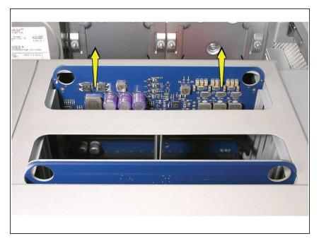
Holding the memory riser card by the two finger holes, pull it out of the memory cage and place the card DIMM side up on a soft, clean cloth.
