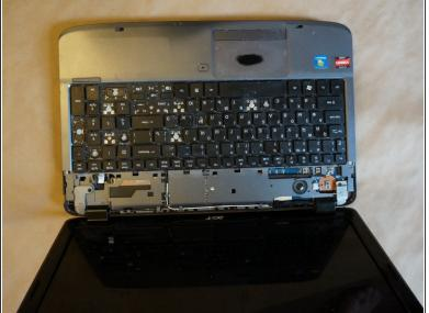
Using plastic openning sticks pick and move up top cover-panel. After disconnectiong all cables put it away.
