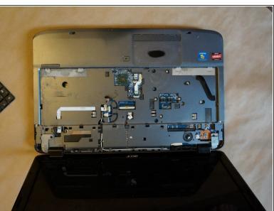
Raise the keyboard a little (slightly bending in order to free its plastic fixtures from the base case).
