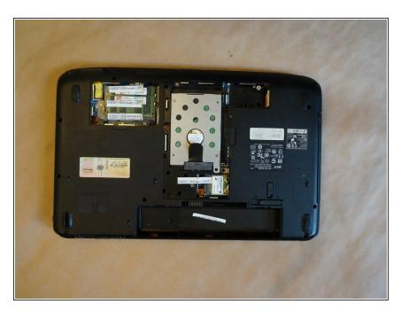
Remove all screws on the bottom of laptop. Remove HD cover (it's not necessary to remove battery and RAM cover)
