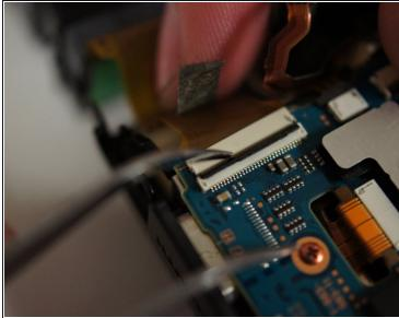
Use the tweezers to lift the black switch on the white receptacle just below the viewfinder. If properly opened, the ribbon cable will remove with very little force.
