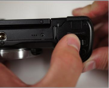
• Close the battery door by pushing it down until it latches shut.
