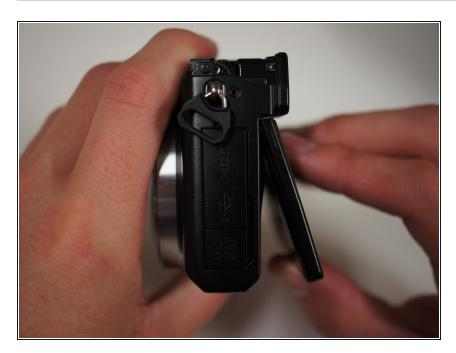
Lift the LCD screen with your fingers such that the screen is bent slightly away from the camera.
