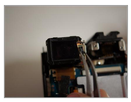
Using the tweezers, unhook the flexible circuit board from the metal tab on the right of the viewfinder by rotating it to the left.
