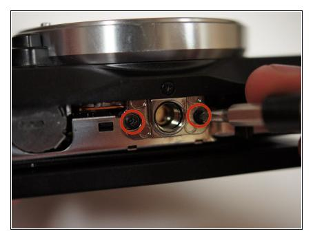
Remove two more 3/32" #00 screws from the bottom of the camera using the Phillips #00 screwdriver.
