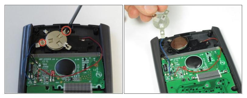
Use a Phillips #00 screwdriver to remove the two 7.5 mm screws holding the battery cover to the case.
