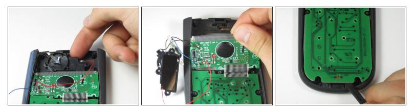
Mhen removing the parts from the calculator be careful not to break any wires or ribbons. The solar panel, screen, and lower circuit board should remain connected throughout this guide.
