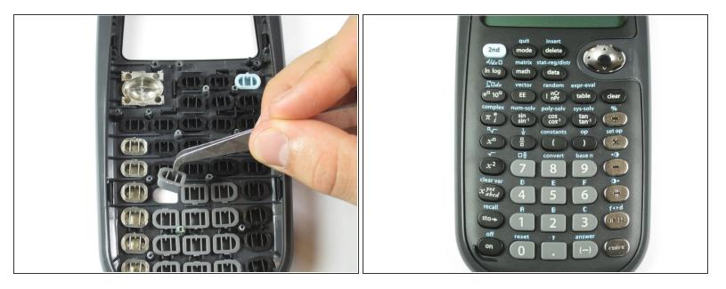
• Locate the button that needs replacement and lift it out of the calculator with tweezers.
