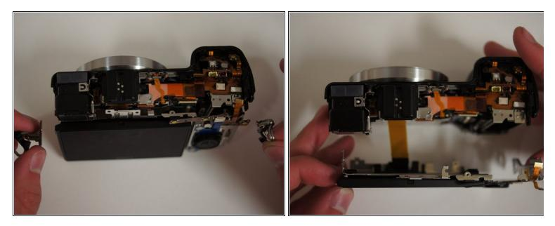
The LCD assembly is attached with a concealed ribbon cable, so be gentle when you remove it.
