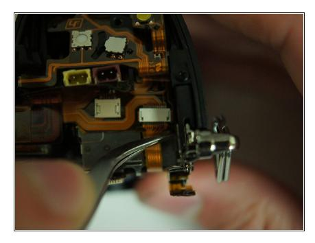
• Unplug the orange ribbon cable on the top right of the camera next to the metal bracket by applying tweezers to the tabs on either side of the plug.
