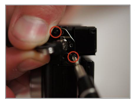
Remove two more 3/32" #00 screws from the metal bracket on the left side of the camera using the Phillips #00 screwdriver.
