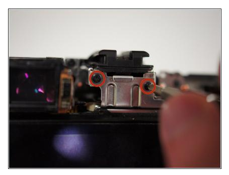
Remove the two 3/32" #00 screws located next to the viewfinder using the Phillips #00 screwdriver.
