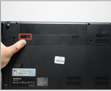
• To unlock the battery, flip the laptop over so that the bottom is facing upward. Then unlock the left clip by pushing the clip to the left.
