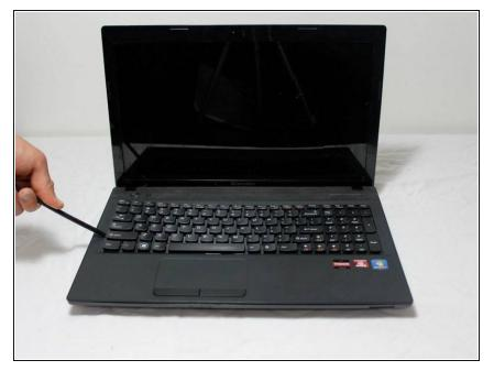
Remove three screws on bottom of case. They have a little keyboard image next to them. If you don't do this first, the keyboard will not come off. Place the plastic spudger right under the edge of the keyboard and lift up the keyboard.
