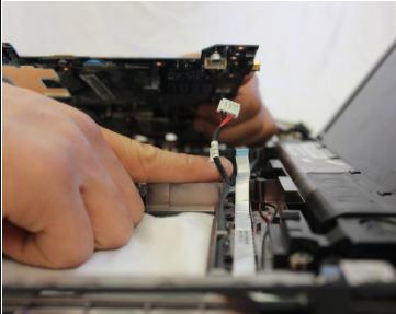
• Remove final plug connecting motherboard to base of laptop.
