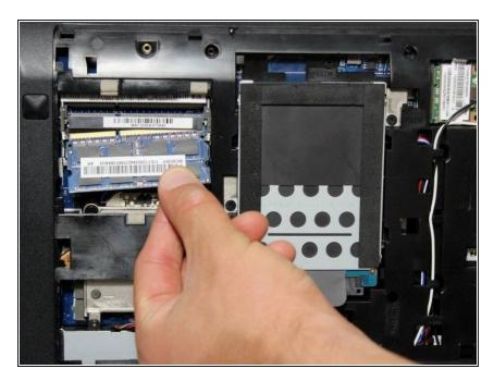
After unlocking the memory from it's position, pull the memory out.
