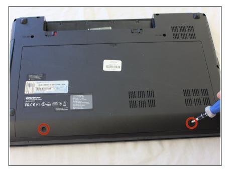
Remove the two screws highlighted.
