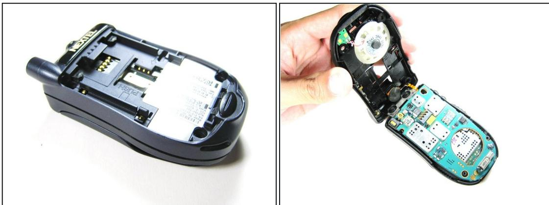
**⚠ DO NOT force the cover off as it could damage the ribbon cable!**
