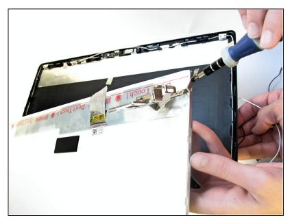
On both sides of the LCD, there will be a screw that attaches the hinges to the display. Use the Phillips #0 screwdriver to unscrew the two 3.2 mm Phillips #0 screws and detach the hinges.
