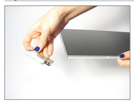
Once the hinge has been unscrewed, remove it from the LCD.
