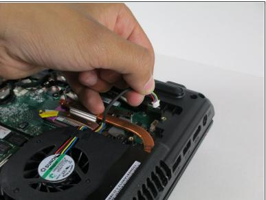
• Disconnect the fan from the motherboard by pulling the black cord straight up.
