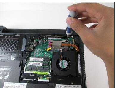
Remove the four 1.25 mm Phillips #1 screw that secure the heat sink in place.
