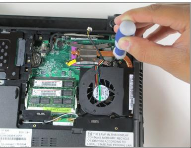
Remove the 1.5mm Phillips #1 screws attaching the fan to the motherboard.
