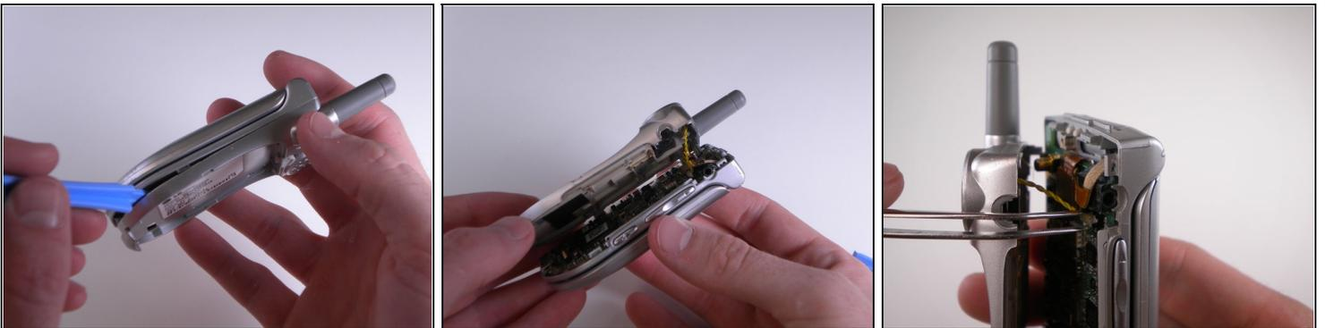
⚠ When removing back cover, be careful not to break the speaker wires.
