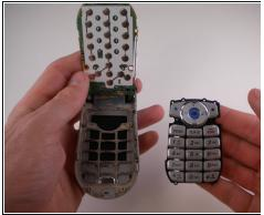
• Use an iPod Opening Tool to lift up on the keypad and pull it out.
