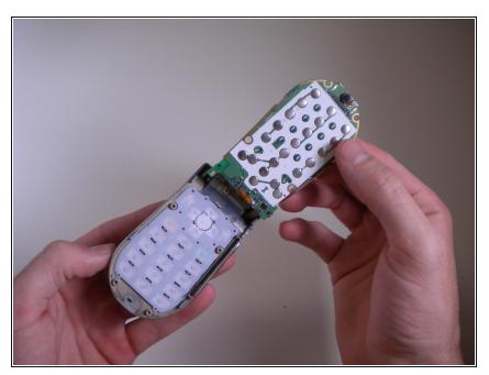
Carefully flip the logic board up and out of the way.
