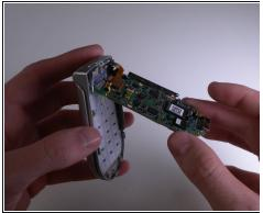
• Carefully pry and lift up on the logic board using an iPod Opening Tool.
