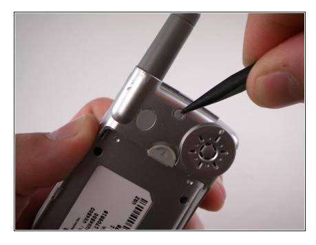
Remove the rubber grommet using a Spudger.
