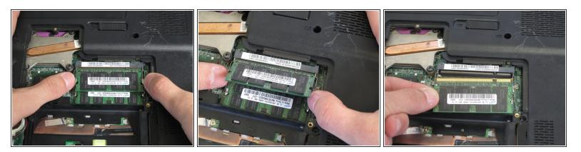
Remove the RAM by placing your thumbs on the silver tabs on each side of the RAM stick and pulling the tabs away from the RAM stick.
