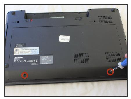
Remove the two screws highlighted.
