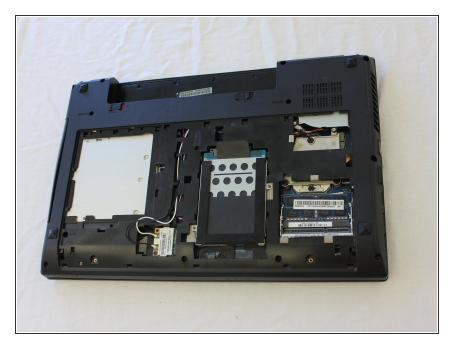
This is the back of the laptop with the cover removed.
