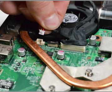
Using two fingers (one on either side of the block) or two plastic opening tools (one on either side of the block), pinch the bottom of the block and lift up to remove the block.
