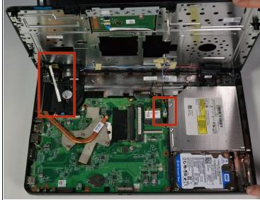
Use a plastic opening tool to pry up the plastic covering of the laptop by wedging it underneath
