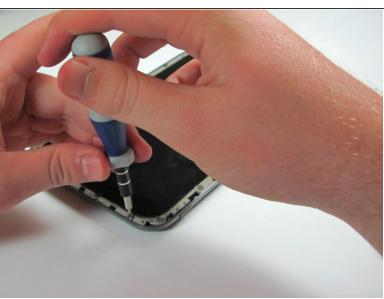
Use a T5 screwdriver to remove the seventeen 5.0 millimeter screws from the back casing.
