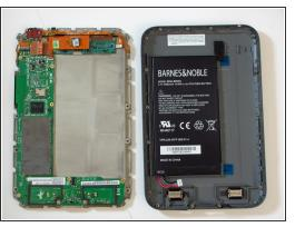
Use the plastic opening tool to gently unclip the wire from the pins by pulling the white connector up.
