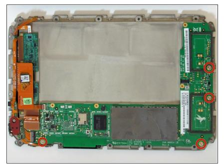
Use the T5 torx screwdriver to remove the four 2.5 millimeter screws that attach the motherboard to the back plate.
